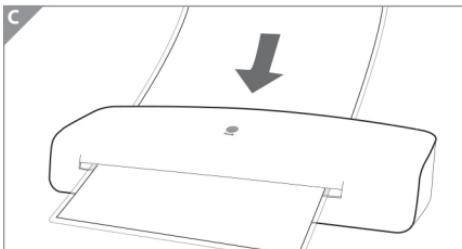
**Insert laminating pouch closed-edge-first into the slot.**
