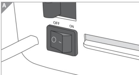
**Move the switch to "ON" to turn the laminator on.**
