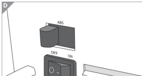
**In case of jammed pouch switch "ABS".**
